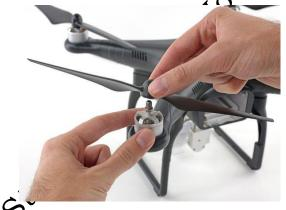
Fig. 1.24 Remove the Propellers
