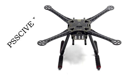
Fig. 1.3 Drone frame and landing gear
